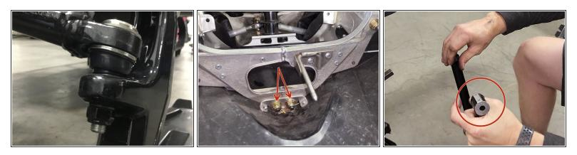
• **IMAGE 1** Now remove the lower ball joint using the same technique you used on the upper ball joint.
